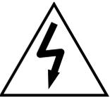
The lightning flash with arrowhead, within an equilateral triangle, is intended to alert the user to the presence of uninsulated “dangerous voltage” within the product’s enclosure that may be of sufficient magnitude to constitute a risk of electrical shock to persons.
