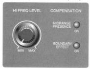
control clockwise increases the high frequency level; turning it counterclockwise reduces the high frequency level.
